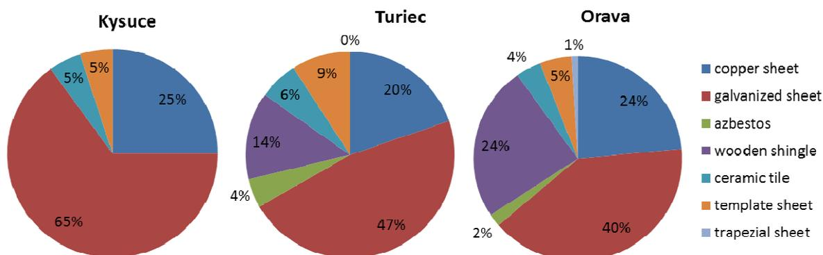
Fig. 6 Representation of roofing types used in selected regions - as a percentage
