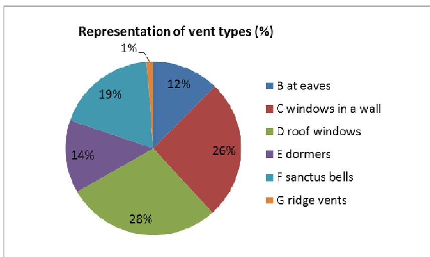
Fig. 4 Various types of vents in selected investigated trusses
