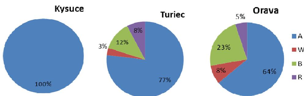
Fig. 7 Representation of floor structure types in selected regions: A - heavy arches, W - wooden arches, B - ceilings of wooden beams, R - ceilings of reinforced concrete
