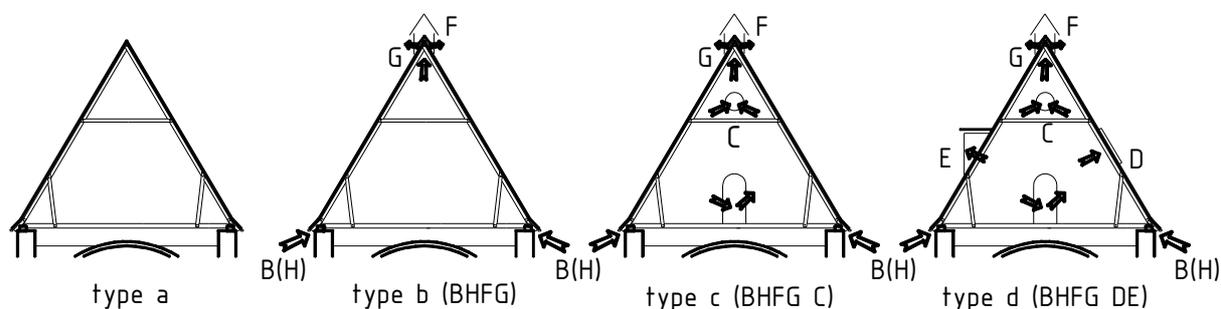
Fig. 3 Basic types of ventilating schemes in under-roof spaces
