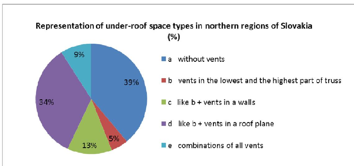
Fig. 5 Individual types of ventilating schemes used for under-roof spaces in historical trusses
