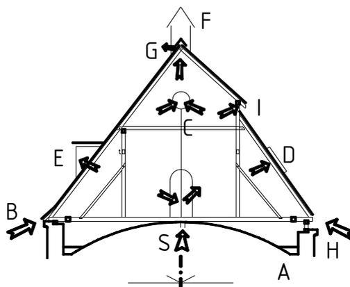
Fig. 2 Openings in the under-roof space of a truss that are essential for space air circulation
